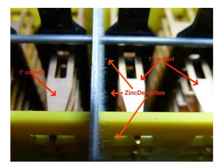
The little whiskers appearing on the zinc-plated metal plate when growing may touch the upper 1' contact blades **and** the 1' upper busbar....
