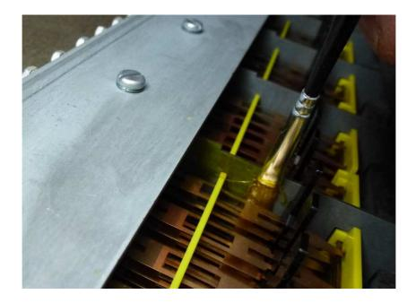
The next picture shows keyboard with metal sides totally coated with yellow protective lacquer.
