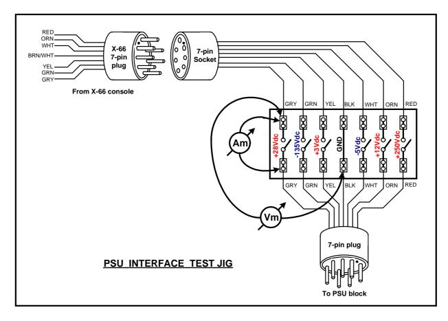
While being quite basic but very helpful, this test jig allows measurements in a simple way of both DC voltages and DC currents.
