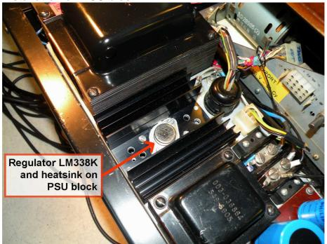
Refer to schematic diagram. Vin of LM338K is connected to the positive terminal of C3 and decoupled by 100 nF capacitor. One elco of 470  $\mu$ F is now sufficient (i.s.o. C5 = 1500  $\mu$ F/50V) at Vout since ripple rejection and regulation is assured by the regulator LM338K. One 100 nF decoupling capacitor is inserted between +28 Vdc output and ground. The role of diodes D13 and D14 is to protect the LM338K regulator as recommended in the datasheet (Fig.3).
