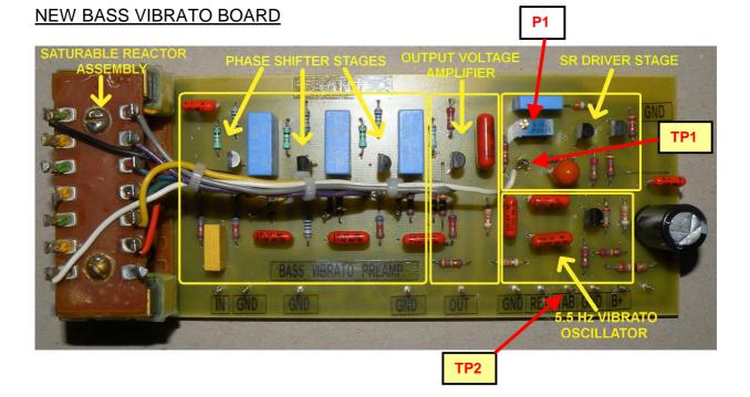
The size of the new board is a replica of the original board and position of connecting points have been taken into consideration to avoid any wiring problem during installation.
