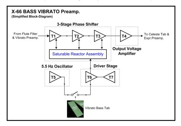
Signals (notes # 1 to # 44) coming from the Flute Filters and pre-amplified by the Vibrato Preamp (refer to schematic diagram Fig 5-7 of the X-66 service manual) are reaching the three series-connected phase shifter stages (T1 to T3).
