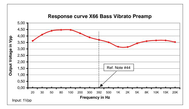
The above graphic depicts the frequency response of the Bass Vibrato circuit from the input up to the output. Since the highest concerned frequency is 392 Hz (note #44), it was expected to get a frequency roll-off from this point onwards.
