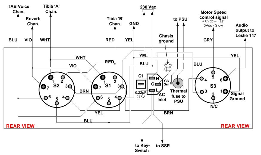
S1: 7 pins socket to TC S2: 7 pins socket to TC
